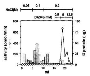
**Fig. 2** Elution profile of PAO activity from 383-Sepharose. The crude enzyme solution ( $200~\mu g$  of protein) was added to the affinity column (0.5~ml). The enzyme was eluted from the column with buffer A containing NaCl and DA343
